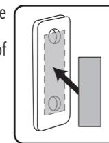
4. Peel off other side of tape adhesive and press firmly for at least 30 seconds in order to make sure the adhesive sticks well to surface.
