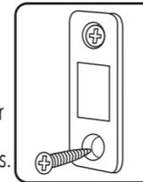
3. Screw the magnetic base and strike plate with screwdriver, ensuring that logo faces out.
