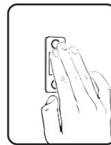
5. Let the adhesive tape cure for at least 24 hours before testing the closure strength.
