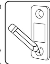
2. Drill pilot holes about the length of each screw at the pencil marks for magnetic base and strike plates.
