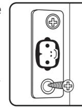
4. Bring magnets together to confirm that they hold together. Adjust as needed.
